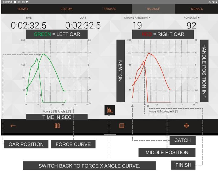
The Force-Curve / Angle-Curve mode works very similarly to the Signals Mode, which is a separate screen and explained a little later in this manual. Per stroke you draw two separate curves per oar handle. One for force over time, one for the handle position over time.
