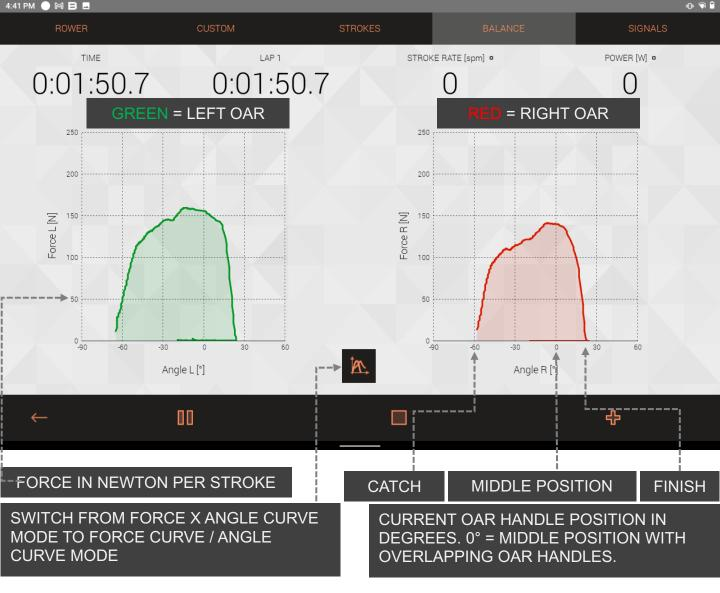
The Balance mode has two views to choose from: how much Force is applied at which position of the stroke or how much force is applied at which point of time with a separate overlayed curve for the oar handle position.
