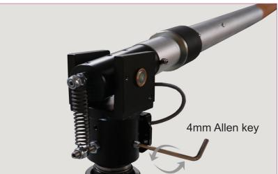
Both oarhandles should be mounted in the maximum catch position, which is approximately 84°. The right piston rod should not be parallel to the outrigger, the left one should. After the oarhandles are placed in the right position, close the Allen screw with an 4mm Allen key on both sides.
