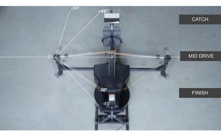
Mid drive position functions as 0°-mark. This is where your oars overlap exactly, or your sweep oar handle is exactly parallel to the outrigger.
