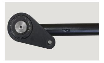
Insert each outrigger **ALL THE WAY** until you feel and hear a solid metal-to-metal noise. The rigger will not go in unless it is held in a vertically and horizontally straight position. The image below indicates how we hold an outrigger to insert it evenly and smoothly.
