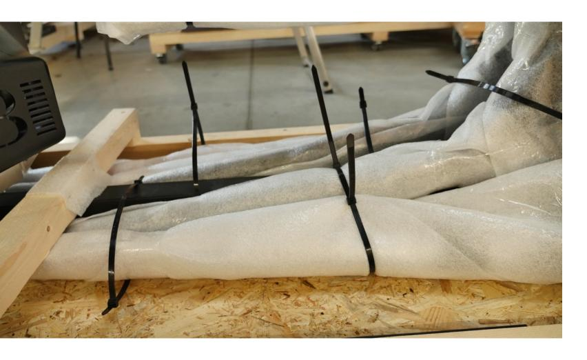
Put zip-ties around the oar-handles (two sculling oar handles, each attached to the oarlock) and one sweep oar-handle. Wrap all zip-ties also around the main body bottom frame. Come through between the main body and the slide frame rail.
