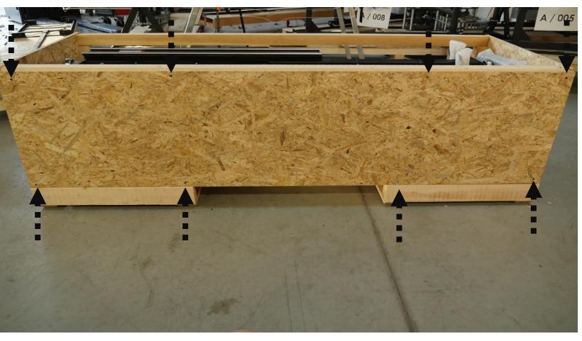
Attach the right side wall with 5x50 screws
