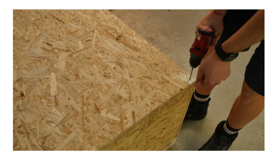
Mount the lid with 5x50 screws, aim to put the screws in the middle of the 50x50 frames below it for maximum hold.
