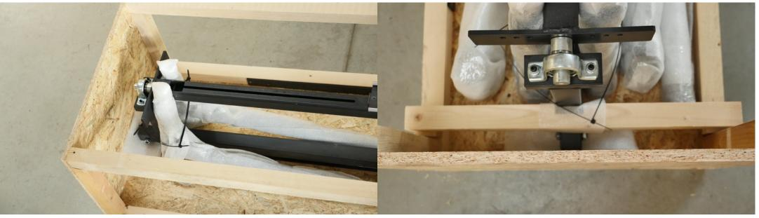
Riggers go in right side up, tie two zip-ties together, go around both riggers and the front (left) part of the main frame. Oar-locks and oar handles are wrapped as one unit (for each side separately) and zip-tied around the bottom part of the
