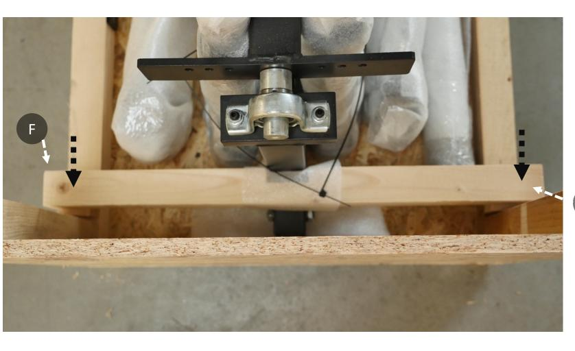
Secure the main body with wrapped part E, use spacers F underneath and 5x12 screws on each side.
