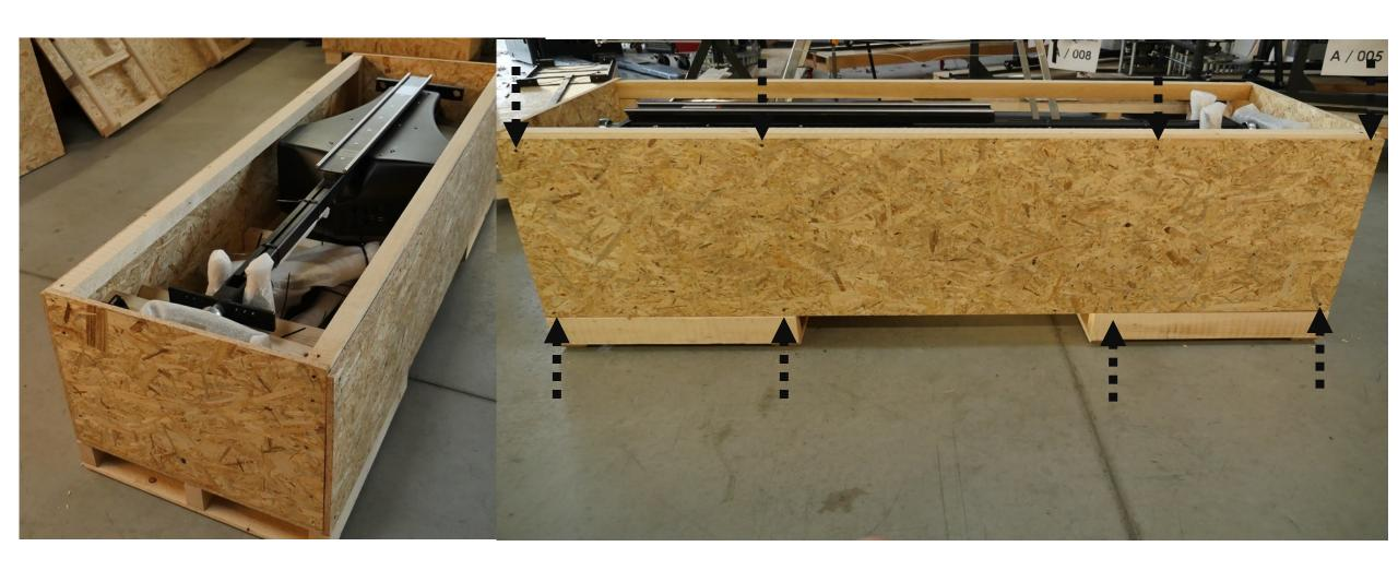
Attach the left side wall with 5x50 screws
